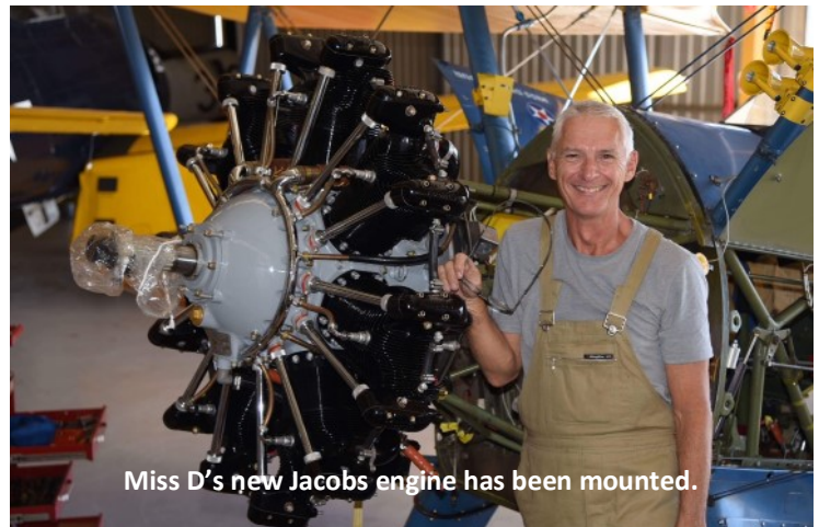
Old Continental in the foreground. New Jacobs being installed by Wayne Milburn of Aerotec Qld Toowoomba.
