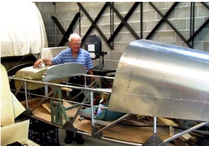
David Archer's Super Diamond takes shape. David has his hand on the long-range fuel tank in the picture on the left above. Story is on Page 10
